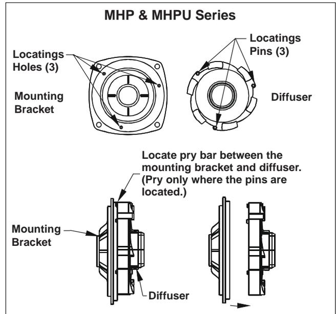
Figure 3. Removing the Diffuser MHP & MHPU Series
