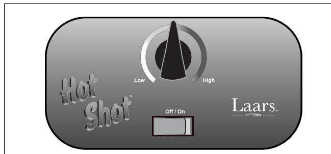
Figure 6. Temperature Control Panel.
