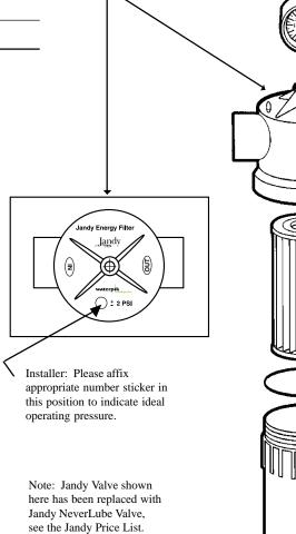
\*Energy Filter Bowls with Lot#1073 and prior, use replacement O-ring part #3179. Lubricate O-ring wth Silicon grease to prevent binding.
